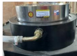
Class 0.5 Accurate load cell
