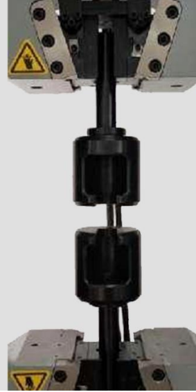
➤Grip for Fasteners (Bolt/Stud/Nut)
