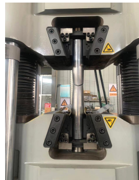
Ad hoc designed half open jaws ensuring easy sample positioning
